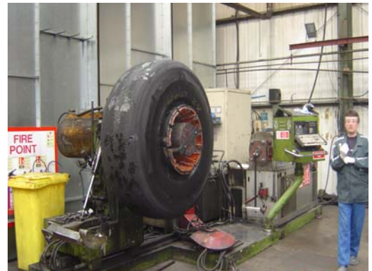
Figure 3 A buffed tyre ready to be retreaded
