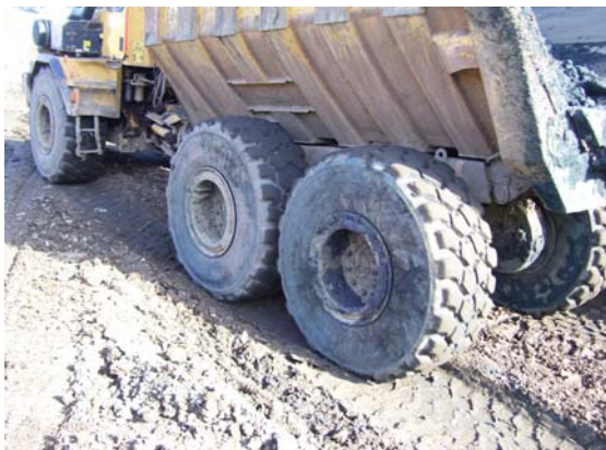
Figure 5 The tyres retreaded with recycled content performed well in tough conditions
